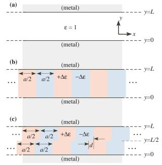
Figure 1: (a) Schematic of a 2d metal waveguide of width L, which supports modes propagating along the x direction. (b) A perturbation  $\pm \Delta \varepsilon$  is introduced via two periodic layers of thickness a/2 filling the waveguide. (c) The perturbation is modified: for half of the thickness  $(y \in [0, L/2])$ , the layers are shifted in the x direction by a distance d.
