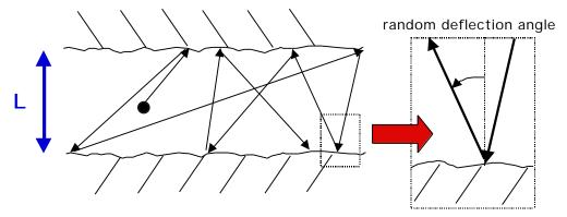
Figure 3. Transport of a gas with Kn>>1 in a rough-walled contained
