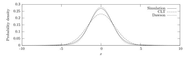
Figure 3: Comparisons between the Central Limit Theorem with and without the Dawson correction, compared to simulations of  $1.6 \times 10^{10}$  walks with N = 3 steps. Even in the central region, the Dawson curve is a better fit to the data.
