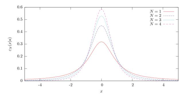
Figure 2: Plots of  $\varepsilon_N(x|a)$  for several different values of N, for the case when a = D = 1. The case of N = 1 is the Cauchy distribution, while the cases N > 1 are from numerical integration of equation 1. The substitution  $1/t = -\log \alpha$  was employed to change the integral into one over a finite range  $0 < \alpha < 1$ , and the resulting expression was evaluated using Simpson's rule.
