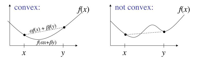
For a convex problem (convex objective & constraints) *any* local optimum *must* be a global optimum ⇒ efficient, robust solution methods available
