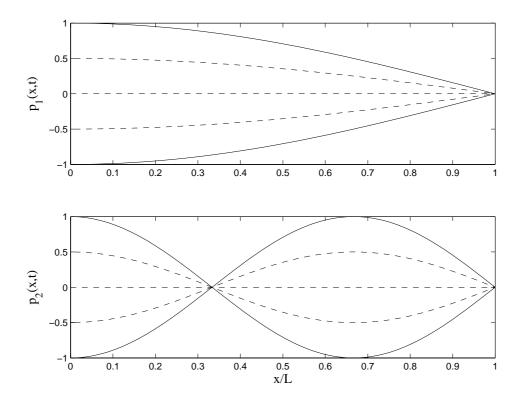
Figure 7: Various phases of the first two normal modes  $p_n(x,t)$  (n = 1, 2) with  $\gamma_n = 1$ . Note that the envelopes (solid lines) are just  $\cos((2n - 1)\pi x/(2l))$ .
