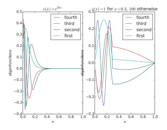
Figure 2: First four eigenfunctions of  $\hat{A}u = (cu')'$  for two different choices of c(x).
