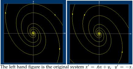
The left hand figure is the original system x' = .6x + y, y' = -x. The right hand figure is the reversed system x' = -.6x - y, y' = x.
