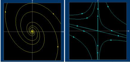
The left hand figure is the original system x' = .6x + y, y' = -1.5x. The right hand figure is the orthogonal system x' = -1.5y, y' = .6x + y.
