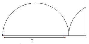
$T = 2\pi \frac{E}{WH}$  is calculated by mesuring the distance between two cusps.
