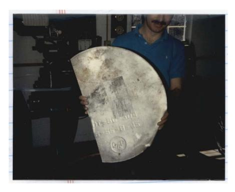
Figure 3: Corroded lid of barrel.
