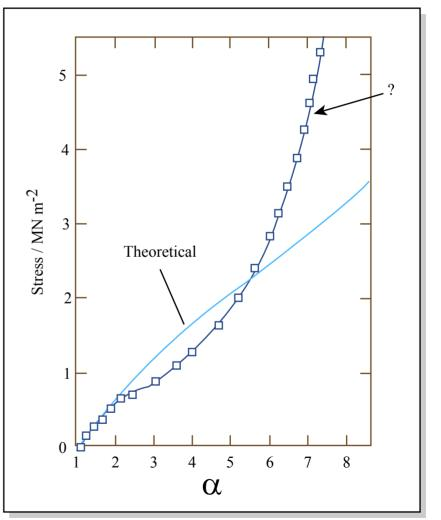
Figure by MIT OCW. High tensile elongations
