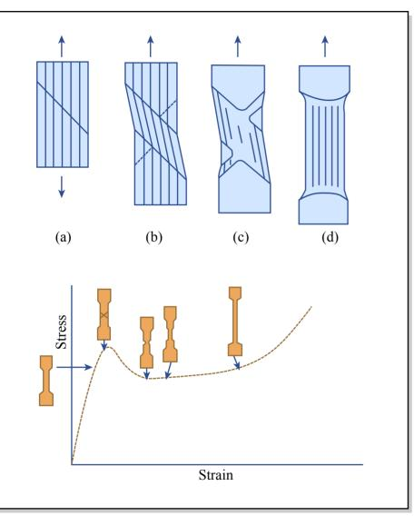
Shear banding in tension or compression.
