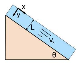
and boundary conditions: at y = 0,  $\frac{dv_x}{dy} = 0$  (no shear) at y = L,  $v_x = 0$  (no slip).
