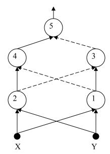
In this network, all the units are sigmoid except unit 5 which is linear (its output is simply the weighted sum of its inputs). All the bias weights are zero. The dashed connections have weights of -1, all the other connections (solid lines) have weights of 1.
