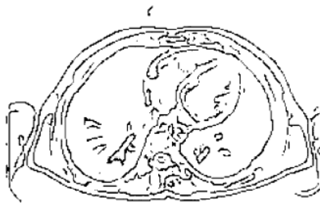
Figure 19. 3D edges after hysteresis thresholding, Shen filter, \alpha = 0.6
