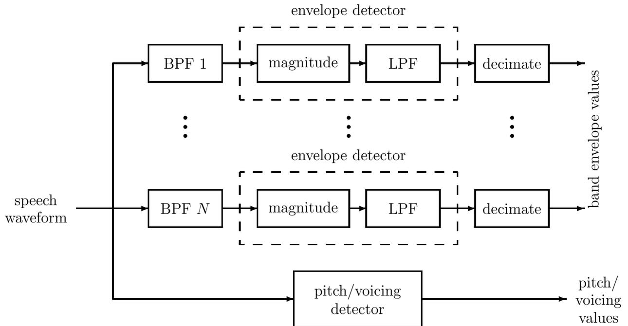
Figure 2: Channel vocoder analyzer
