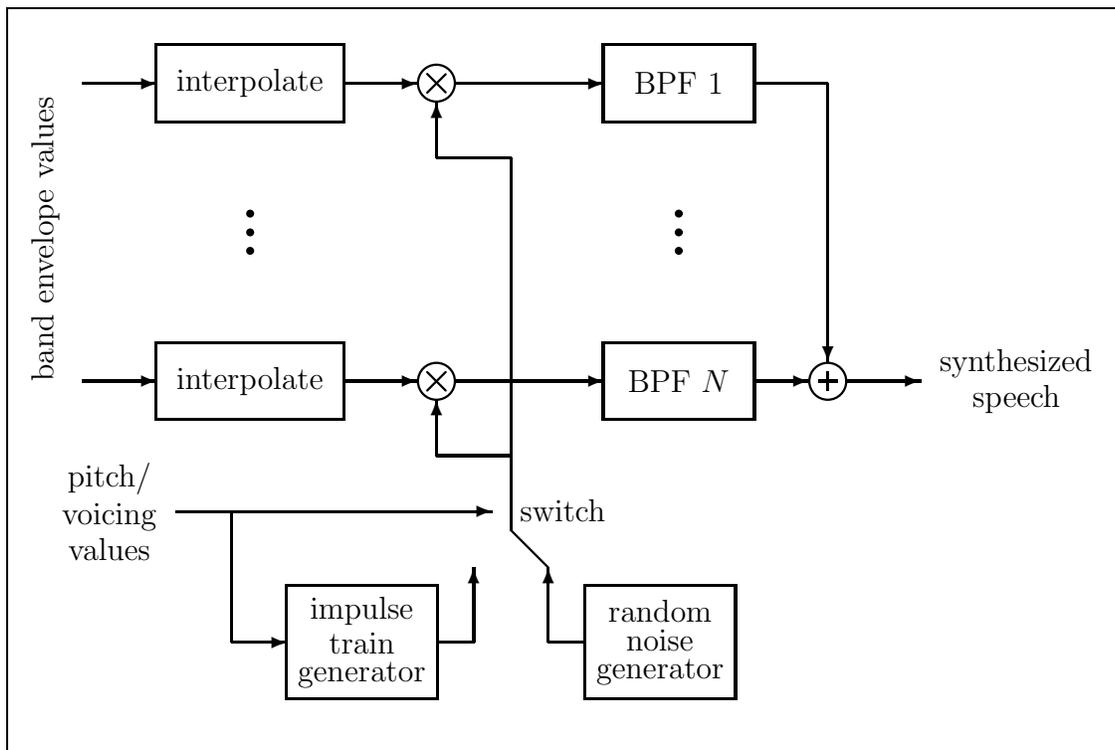
Figure 3: Channel vocoder synthesizer
