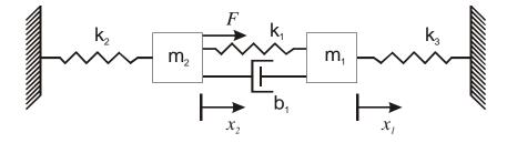
In the  $e \rightarrow V$  convention, the flows are the time derivatives of the displacements  $x_i$  of the different bodies, and effort is the external force. Since  $k_1$  and  $b_1$  share the same displacement, and hence, the same flow, they are in series. The same holds for  $k_2$  and  $m_2$  and also for  $k_3$  and  $m_1$ . By observation, the net flow through  $b_1$  is  $(\dot{x}_2 - \dot{x}_1)$ . Hence, the equivalent circuit can be represented as shown in Figure.
