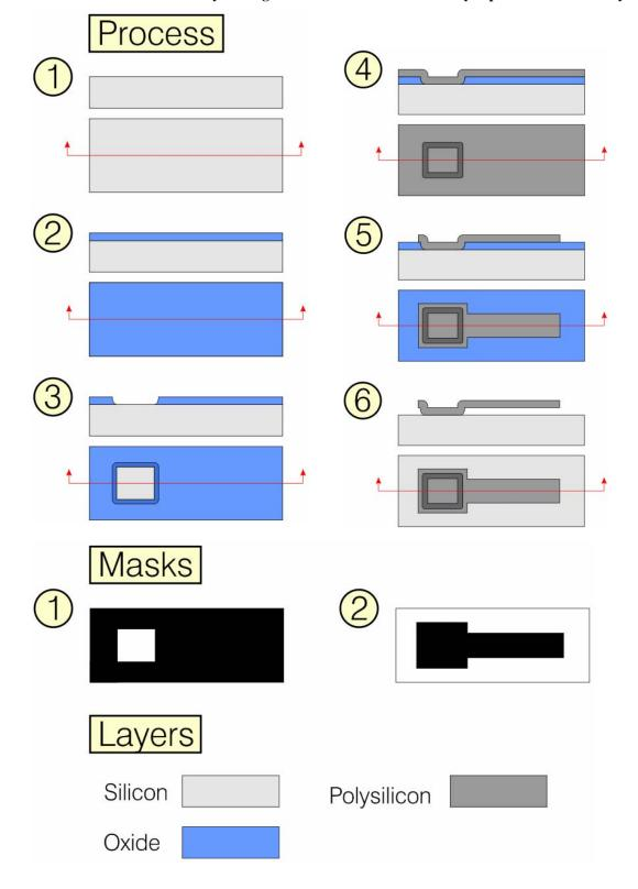
6. Release the cantilever by etching the oxide with BOE followed by super-critical freeze drying.
