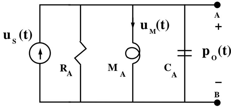
Figure 3: Example of an acoustic circuit consisting of a volume velocity source, an acoustic mass, an acoustic resistance, and an acoustic compliance connected in parallel. All pressures and volume velocities are assumed to have the same  $e^{st}$  time dependence, i.e.  $u_S(t) = U_S e^{st}$ ,  $u_M(t) = U_M e^{st}$ , and  $p_O(t) = P_O e^{st}$ .
