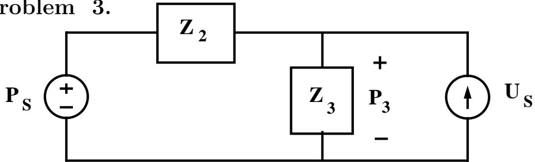
Figure 2: An acoustic circuit consisting of a pressure source, a volume velocity source and two impedances. All pressures and volume velocities are assumed to have the same  $e^{st}$  time dependence.
