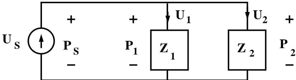
Figure 1: Example of an acoustic circuit consisting of a volume velocity source and two elements connected *in parallel*. All pressures and volume velocities are assumed to have the same  $e^{st}$  time dependence.
