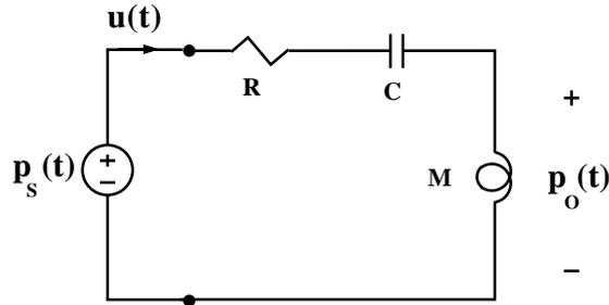
Figure 4: Example of an acoustic circuit consisting of a pressure source, an acoustic mass, an acoustic resistance, and an acoustic compliance, all connected in series. All pressures and volume velocities are assumed to have the same  $e^{st}$  time dependence.
