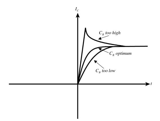
Real circuits do exactly this!  $C_B$  may require some trimming, but this is a trick that works in the real world.
