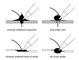
Figure 4.1: Good and bad soldering technique
