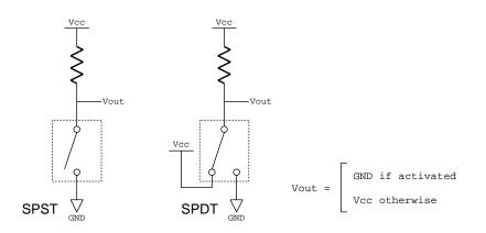
Figure 5.1: Digital Sensor Circuit
