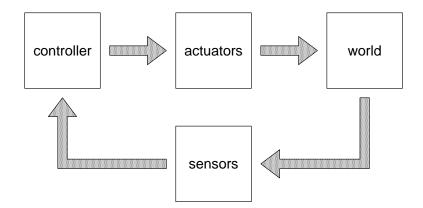
Figure 7.3: Closed loop (feedback) information flow
