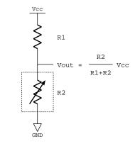
Figure 5.3: Resistive Analog Sensor Circuit
