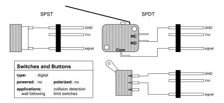
Figure 5.2: Switches and buttons
