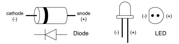
Figure 4.5: Identifying diode leads
