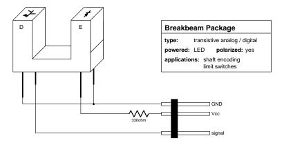
Figure 5.7: Breakbeam sensor package
