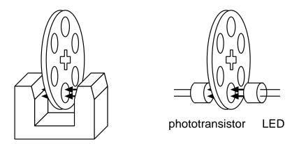
Figure 7.8: Shaft encoding using a LEGO pulley wheel
