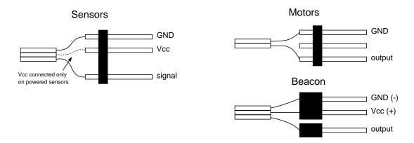
Figure 4.7: 6.270 connector standard
