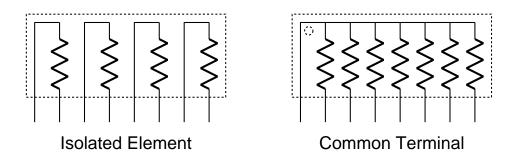
Figure 4.4: Resistor pack internal wiring
