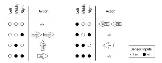
Figure 7.7: Line following with 3 reflectance sensors
