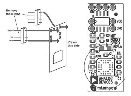
Figure 1. Gyro board showing axis of rotation and connections.
