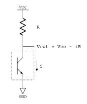
Figure 5.5: Transistive Analog Sensor Circuit
