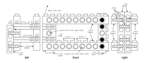
Figure 4.8: Jig for motor assembly
