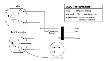
Figure 5.6: LED and Phototransistor
