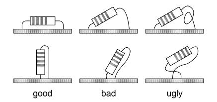
Figure 4.2: Axial component mounting
