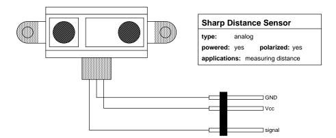
Figure 5.8: Sharp Distance Sensor
