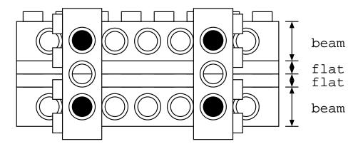
Figure 6.2: A Simple Braced Structure
