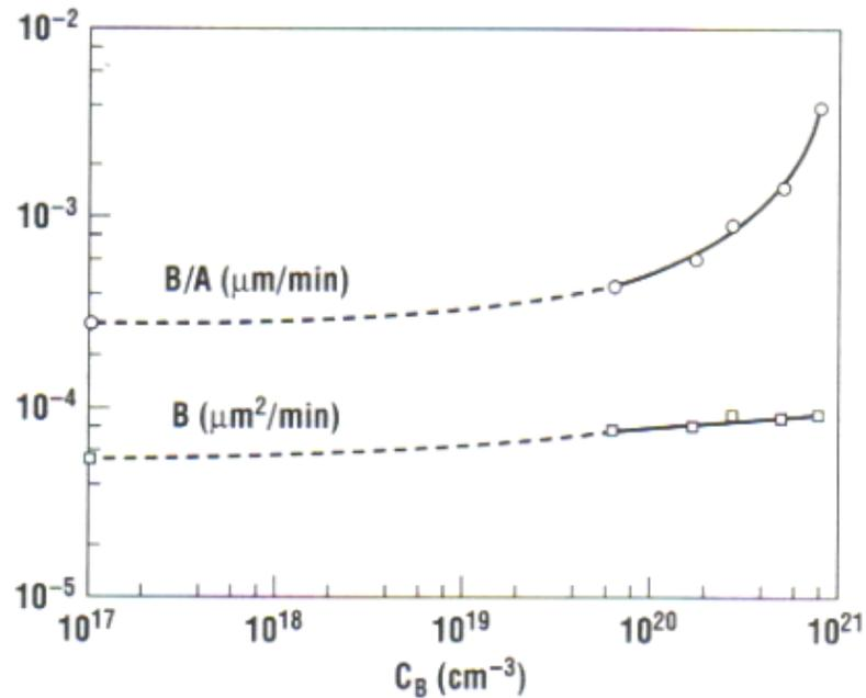
The linear rate,  $B/A$ , rises rapidly because the doping causes an enhancement in the surface reaction rate. The parabolic rate,  $B$ , rises slightly, which would be a result of an increase in diffusion of oxidant through the oxide as a result of the dopant changing the silicon dioxide.
