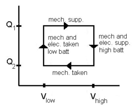
Figure 10–5: Charging Cycle energy movement
