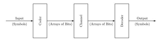
Figure 3.1: Generalized communication system
