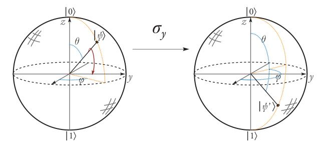
Figure 13.4: Operation of  $\sigma_y$ , on the Bloch sphere
