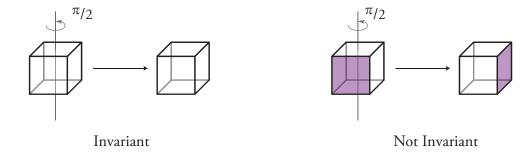
Figure 13.3: Concept of invariance. Symmetry operation: rotation of  $\pi/2$  about the vertical axis.
