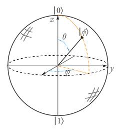
Figure 13.2: Geometrical representation of a Qubit: Bloch Sphere
