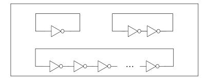
Figure 1.3: Some sequential logic circuits
