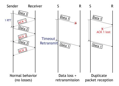
Figure 19-1: The stop-and-wait protocol. Each picture has a sender timeline and a receiver timeline. Time starts at the top of each vertical line and increases moving downward. The picture on the left shows what happens when there are no losses; the middle shows what happens on a data packet loss; and the right shows how duplicate packets may arrive at the receiver because of an ACK loss.
