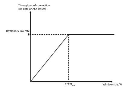
Figure 19-8: Throughput of the sliding window protocol as a function of the window size in a network with no other traffic. The bottleneck link rate is B packets per second and the RTT without any queueing is RTT<sub>min</sub>. The product of these two quantities is the bandwidth-delay product.
