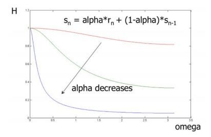
Figure 19-4: Frequency response of the exponential weighted moving average low-pass filter. As  $\alpha$  decreases, the low-pass filter becomes even more pronounced. The graph shows the response for  $\alpha=0.9,0.5,0.1$ , going from top to bottom.
