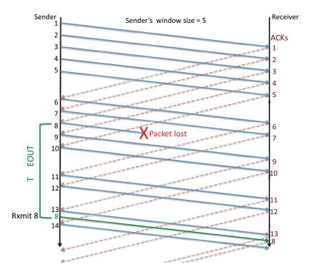
Figure 19-7: The sliding window protocol in action (W=5 here).
