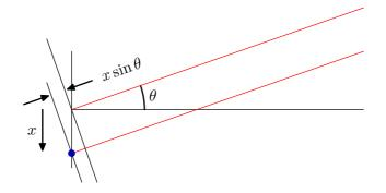
Phase at a point x is delayed (i.e., negative) relative to that at 0:
