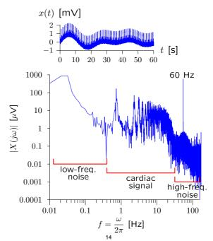
Filter design: low-pass flter + high-pass filter + notch.
