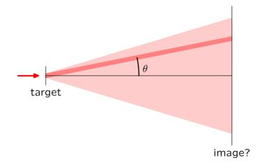
The phase of light scattered from different parts of the target undergo different amounts of phase delay.
