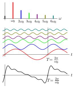
Only periodic signals: all harmonics of  $\omega_0$  are periodic in  $T=2\pi/\omega_0$ .
