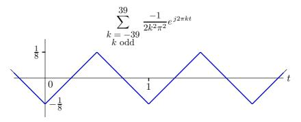
Fourier series representations of functions with discontinuous slopes converge toward functions with discontinuous slopes.
