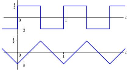
Therefore the Fourier coefficients of the triangle waveform are  $\frac{1}{j2\pi k}$  times those of the square wave.
