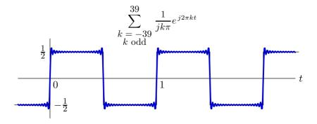
Partial sums of Fourier series of discontinuous functions "ring" near discontinuities: Gibb's phenomenon.
