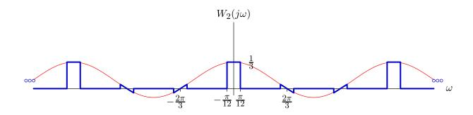
The signal  $w_2(t)$  can be derived by convolving  $w_1(t)$  with a signal
