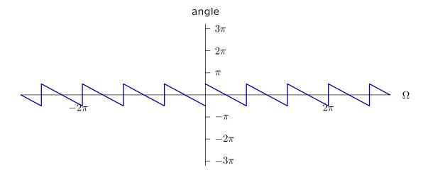
$$H(e^{j\Omega}) = 1 - e^{-j3\Omega} = e^{-j3\Omega/2} \left( e^{j3\Omega/2} - e^{-j3\Omega/2} \right) = j2e^{-j3\Omega/2} \sin \frac{3\Omega}{2}$$
