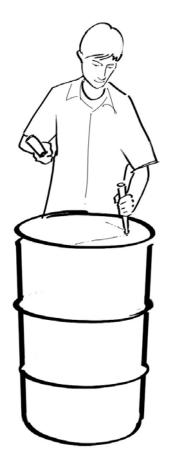
Cut a large opening for filling the kiln with the material you want to carbonize.
