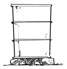
Before starting the burn, place the drum on top of three stones, so that air can flow through the holes in the bottom.
