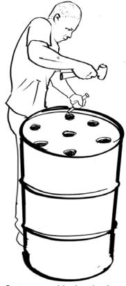
Cut several holes in the bottom of the drum. These holes allow air to flow through the drum while burning, which results in a hotter fire and produces better charcoal.
