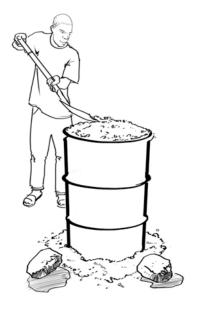
Seal the bottom edges and the top of the drum with sand or dirt to prevent oxygen from entering. Wait at least 2 hours before opening.
