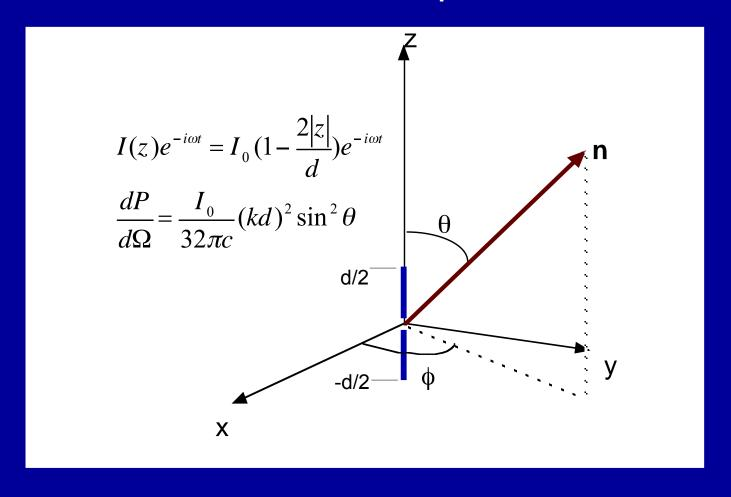
P is the radiated power from the antenna, with current I<sub>0</sub> center fed into antenna
