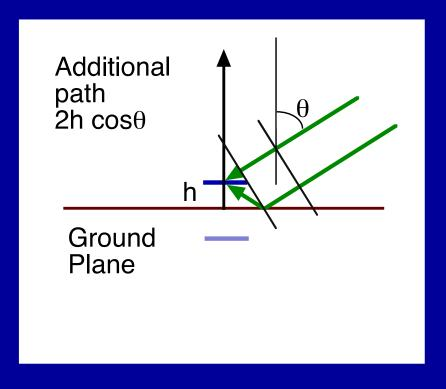
If the ground plane is infinite, then antenna acts like a point source, in the ground plane below the antenna.
