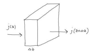
If there are neither sources nor sinks of heat, then a net heat flow into the slab must change its temperature (i.e., energy is conserved).
