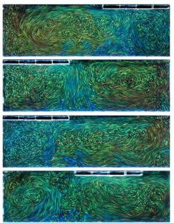
Here the viscous flow moves the floating boundary and the the boundary affects the flow, an interplay roughly analogous to fluid motions beneath tectonic plates.
