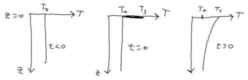
(Note that in the seafloor problem, the half-space will be cooled from above, so that  $T_s < T_0$ , but the mathematical development is unchanged.)
