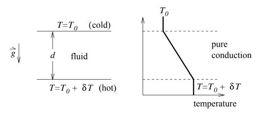
In the absence of convection—the transport of hot fluid up and cold fluid down—the temperature gradient is constant.
