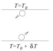
Left undisturbed, buoyancy forces would allow the hot blob to continue rising and the cold blob to continue falling.
