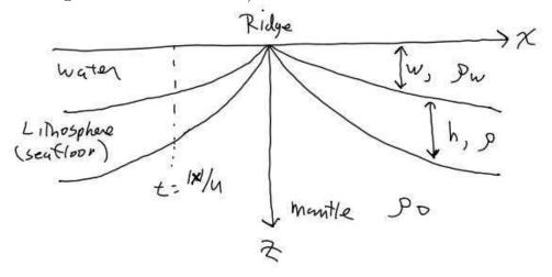
The seafloor (i.e., oceanic lithosphere) thickens as it cools, because underlying hot mantle material is converted to lithosphere.
