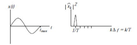
We calculate the power spectrum analytically, beginning with the DFT:
