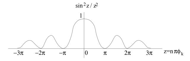
The plot gives the kth component of the power spectrum of  $e^{i2\pi t/T}$  as a function of  $\pi(t_{\text{max}}/T - k)$ .
