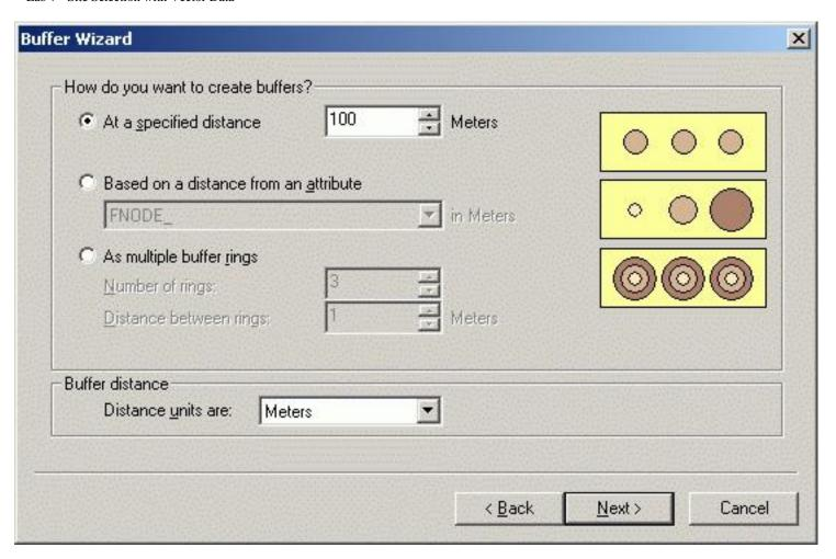
Click Next. The output from a buffer operation can be a shapefile or a graphic on the map. We want to create a shapefile. In the next window (below), select "In a new layer...", and define the output location as your Lab8 folder. Name the file "trains\_buffer", as shown below.
