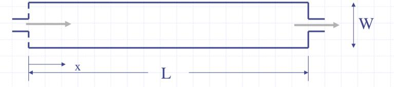
Engineer delayed response (--> plug flow) by making the reactor long & narrow. Density stratification should also be minimal (see Sect 5.4.1)
