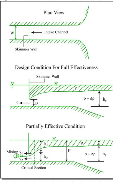
Selective withdrawal of water from density stratified tank or reservoir
