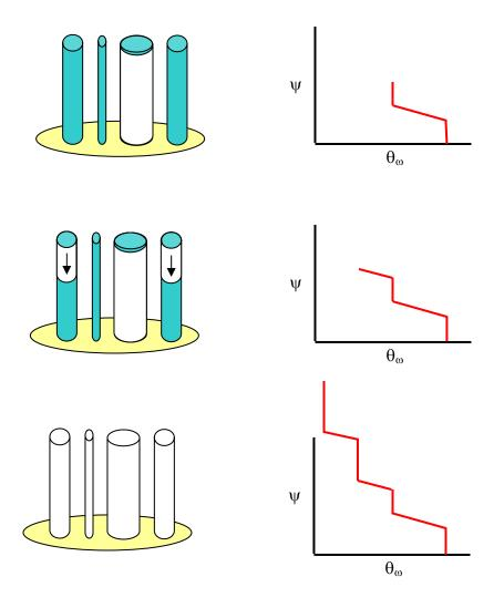
Pore space in rocks and soil is much more complex geometrically but analogous phenomena give rise to characteristic retention curves for a given sample material.
