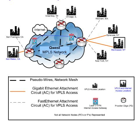
Figure 1 –Qwest iQ Networking Enhanced Ethernet Port Solution for TacDoh Corporation
