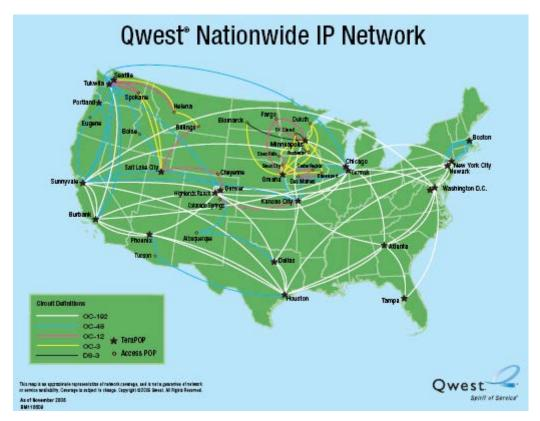
Figure 2 – Qwest's iQ Networking IP Network
