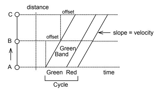
The *slope* of the line defining the green band is speed (the ratio of distance to time). If a car stays within that green band as it goes through traffic signals A, B and C, it will continue unopposed by a red light.
