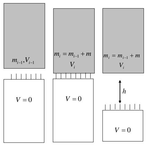
Before Collision After Collision  Linear Momentum before collision
