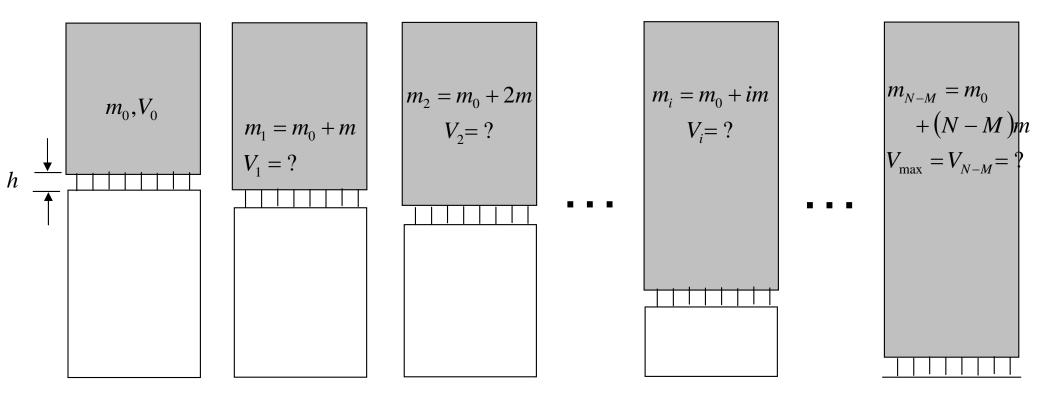
Sequence of 1-story free-falls: when mass collides with floor below, they continue together the free fall until next floor level. There is no resistance to this fall (neither Strength, drag force, etc...)
