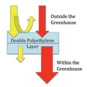
**Figure 3** The effect of double polyethylene layer on incoming radiation. The red arrows represent diffuse radiation that is magnified by the glazing. The yellow arrows are direct radiation, some of which is reflected at the surface.
