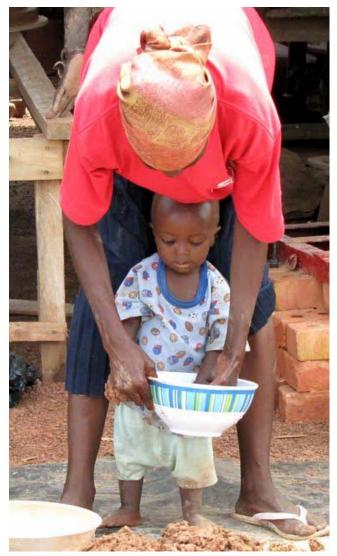
6. Measuring and adding water to clay mixture
