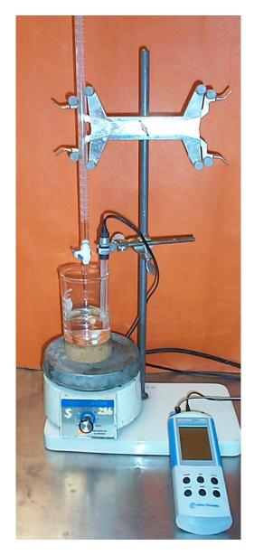
Fig. 3. Titration apparatus: 400-500-mL beaker, 1" stir bar, 25-mL buret, magnetic stirrer, cork, electrode connected to Accumet AP61 pH meter.
