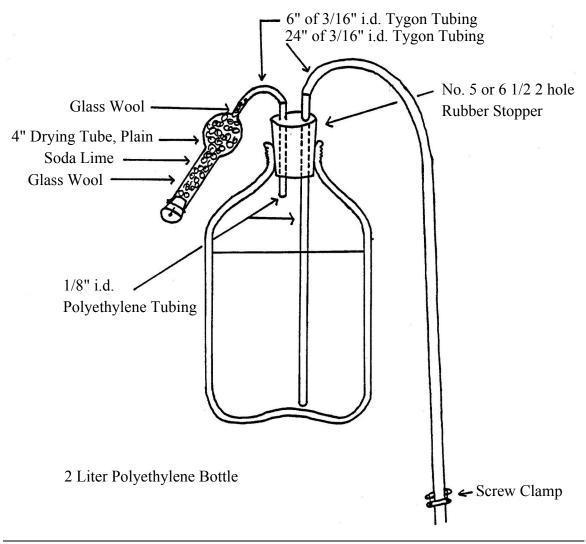
Fig. 1. Siphon storage bottle for standard NaOH
