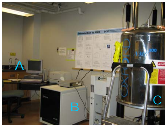
Figure 1 NMR Equipment: (A) Computer Workstation, (B) NMR Console, generates and receives RF, (C) NMR Magnet.
