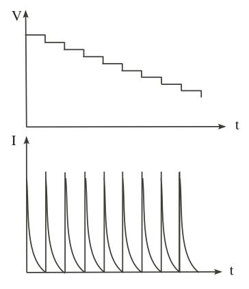
Figure 5: The input voltage steps and current response, which goes as  $\sqrt{\frac{D}{t}}$ , are shown for PITT.  $D(c_0)$  can be inferred from such measurements.
