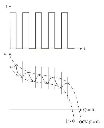
Figure 3: GITT: The dashed curves indicate the open-circuit voltage and the voltage response for some fixed I > 0 respectively.
