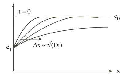
Figure 4: If we fix the concentration at the boundary to be  $c_1$ , we observe how the current responds in time.
