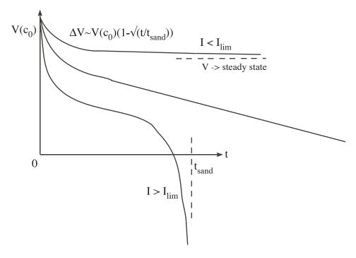
Figure 2: V(t) for values of suddenly applied  $I < I_{lim}$ ,  $I = I_{lim}$  and  $I > I_{lim}$  respectively. For small times,  $\Delta V \sim V(c_0) \left(1 - \sqrt{\frac{t}{t_{sand}}}\right)$ . For large times,  $I < I_{lim}$  leads to a steady state voltage;  $I = I_{lim}$  leads to a voltage hitting 0; and  $I > I_{lim}$  diverges logarithmically at Sand's time.
