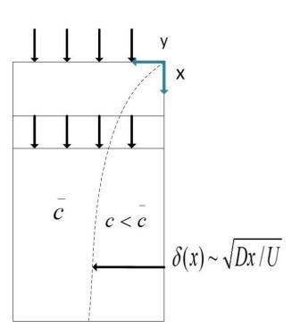
Figure 1: Plug flow through inert porous media
