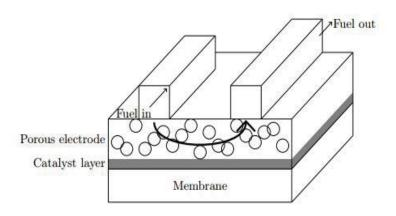
Figure 3: Membrane-electrode assembly
