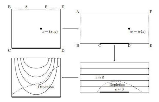
Figure 5: Solving the convection-diffusion problem using conformal mapping
