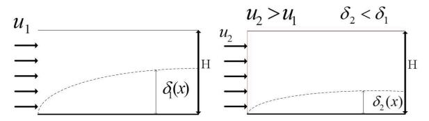
Figure 6: Convective flow of fluid over a reacting surface
