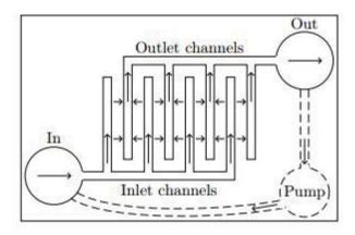
Figure 4: Interdigitated flow channels
