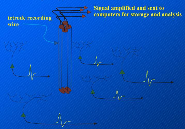
Multiple tetrode recording bundles can be combined into an adjustable array, allowing for up to 150 cells to be monitored simultaneously.
