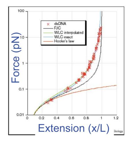
Force versus extension data (red crosses) for  $\lambda$  phage dsDNA (48,502 bp) pulled by magnetic beads in 10 mM Na<sup>+</sup> buffer [4]. The data are fit to a WLC model solved numerically (WLC exact) or using Equation 3 (WLC interpolated), both assuming P = 53 nm. The FIC curve assumes b = 2P = 106 nm. The Hooke's law force curve is from Equation 2.
