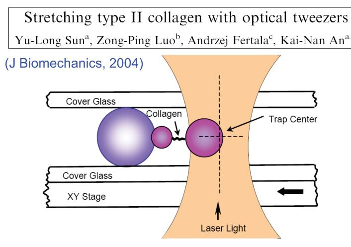
Fig. 1. Stretching a single collagen molecule using optical tweezers. One end of collagen is attached to the bead trapped by optical tweezers. The other end is attached to the small bead fixed with a big bead, which is clamped with two cover glass. Before collagen is stretched, the small bead and the trapped bead are touched. The
