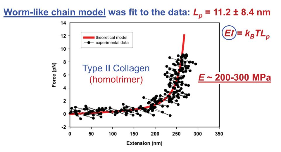
Fig. 2. The force-extension curve for stretching a single type II collagen molecule. The data were fitted to Marko–Siggia entropic elasticity model. The molecule length and persistence length of this sample is 300 and 7.6 nm, respectively.
