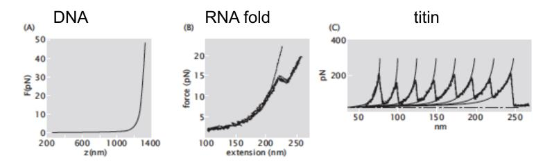
Figure 8.23: Force-displacement curve for a variety of different molecules illustrating the sense in which single molecule experiments serve as the basis of force spectroscopy.
