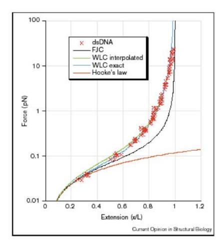
Force versus extension data (red crosses) for  $\lambda$  phage dsDNA (48,502 bp) pulled by magnetic beads in 10 mM Na<sup>+</sup> buffer [4]. The data are fit to a WLC model solved numerically (WLC exact) or using Equation 3 (WLC interpolated), both assuming P = 53 nm. The FJC curve assumes b = 2P = 106 nm. The Hocke's law force curve is from Equation 2.
